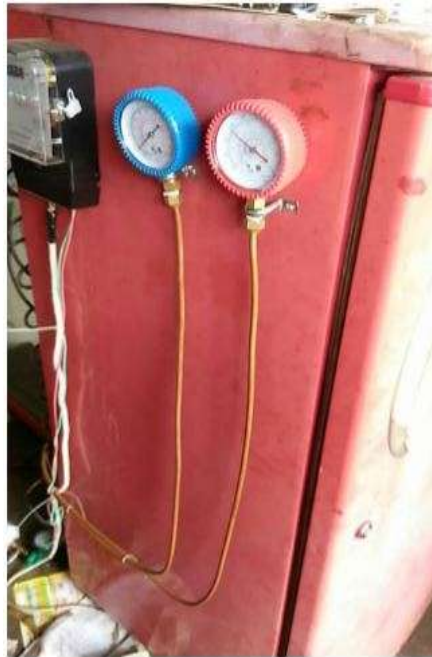
Fig.5 Refrigerator connected with pressure gauges and energy meter
