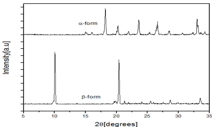
Figure 2. Crystal structure of  $\alpha$ -form and  $\beta$ -form crystal product
