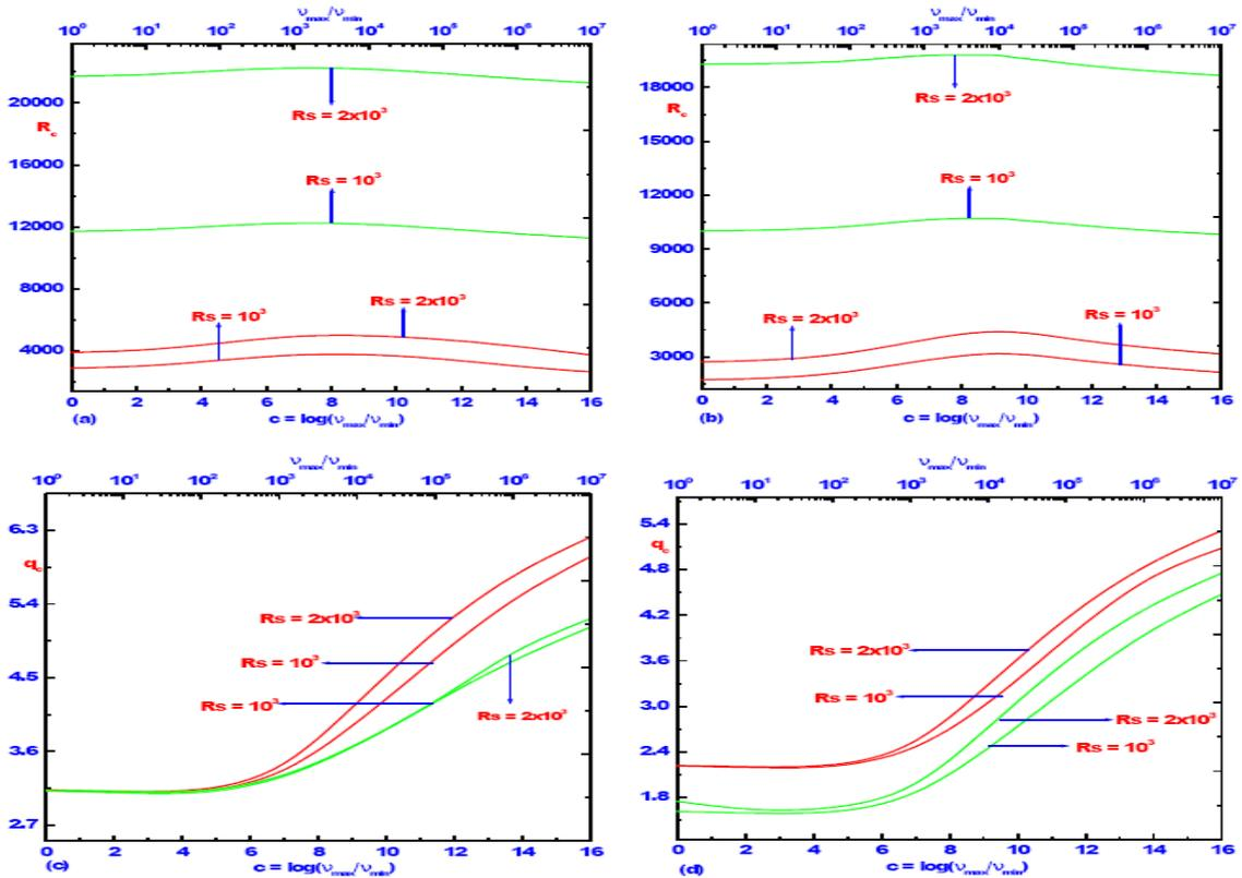
**Figure 5:** Critical Rayleigh number  $R_c$  and critical wave number  $q_c$  versus viscosity ratio  $c$  for  $L = 0.1$  and  $Pr = 10^3$ . Figs. (a) and (c) are plotted for  $R/R$  boundaries. Figs. (b) and (d) are plotted for  $F/F$  boundary conditions. Green and red lines are corresponding to stationary and oscillatory convections, respectively.
