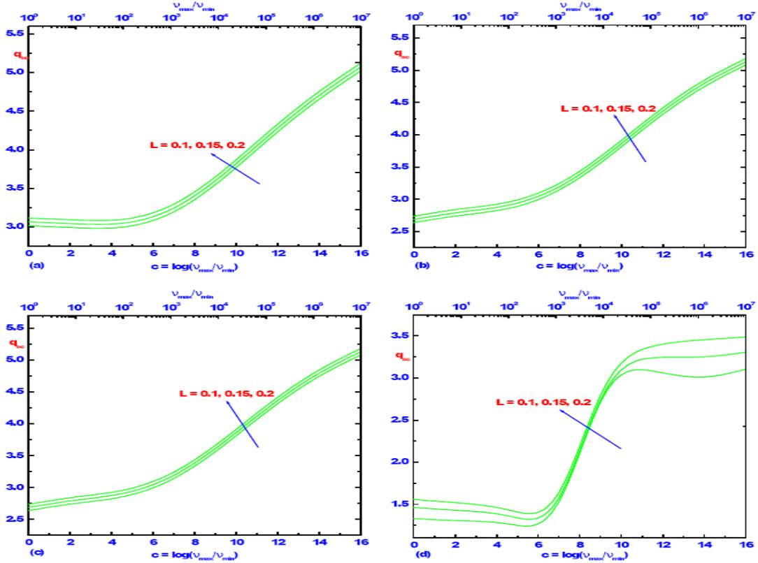
**Figure 4:** The effect of Lewis number  $L$  and viscosity ratio  $c$  on  $q_{sc}$  for  $R_s = 5 \times 10^3$ . Numerically plotted neutral stability curves to represent onset of stationary convection for exponential fluid. Figure 4(a-d) are plotted for  $R/R$ ,  $R/F$ ,  $F/R$  and  $F/F$  boundary conditions respectively.
