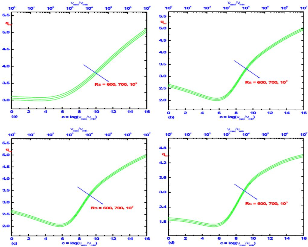
**Figure 2:**The effect of  $R_s$  and  $c$  on  $q_{sc}$  for  $L = 0.1$  and  $P_7$ . Numerically plotted neutral stability curves to represent onset of stationary convection for exponential fluid. Figure 1(a-d) are plotted for  $R/R$ ,  $R/F$ ,  $F/R$  and  $F/F$  boundary conditions respectively.
