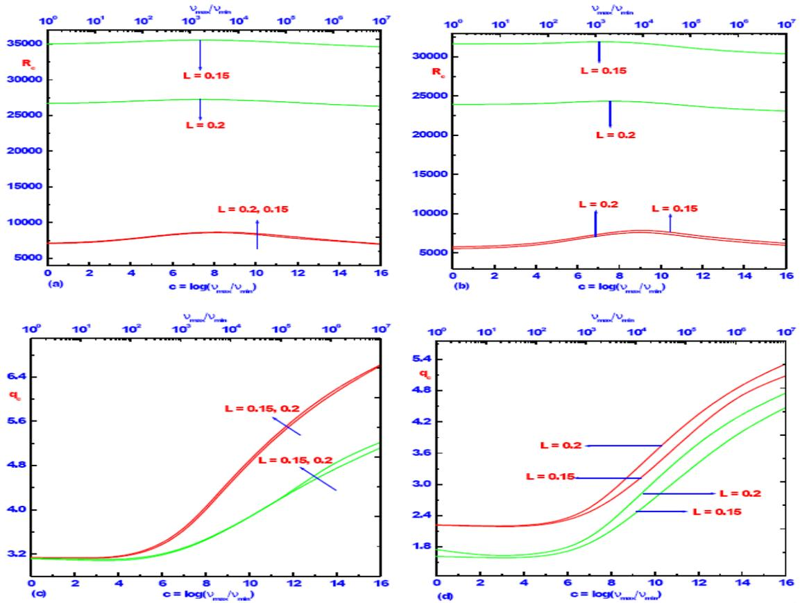
**Figure 6:** Critical Rayleigh number  $R_c$  and critical wave number  $q_c$  versus viscosity ratio  $c$  for  $R_s = 5 \times 10^3$  and  $Pr = 10^3$ . Figs. (a) and (c) are plotted for  $R/R$  boundaries. Figs. (b) and (d) are plotted for  $F/F$  boundary conditions. Green and red lines are corresponding to stationary and oscillatory convections, respectively.
