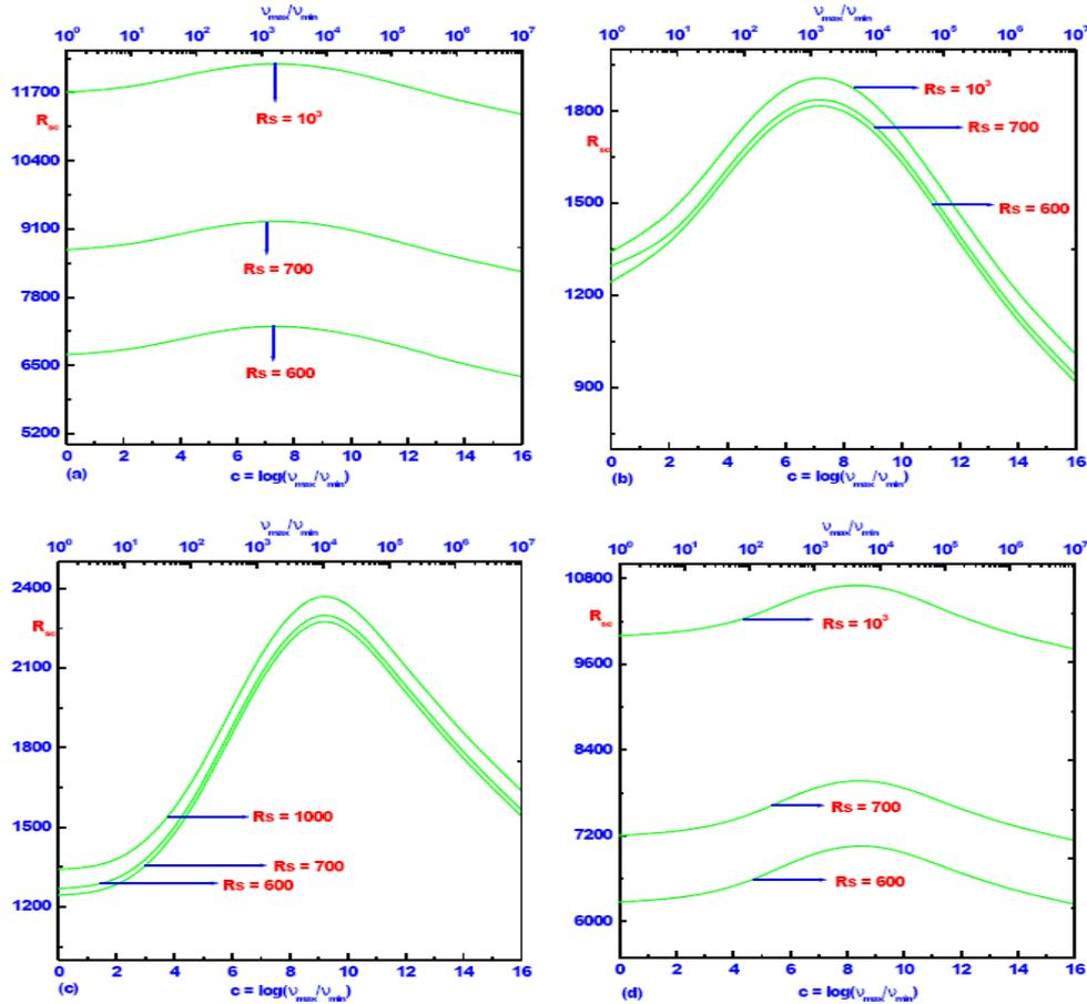
**Figure 1:** The effect of  $R_{sc}$  and  $c$  on  $R_{sc}$  for  $L = 0.1$  and  $P_r$ . Numerically plotted neutral stability curves represent onset of stationary convection for exponential fluid. Figure 1(a-d) are plotted for  $R/R$ ,  $R/F$ ,  $F/R$  and  $F/F$  boundary conditions respectively.
