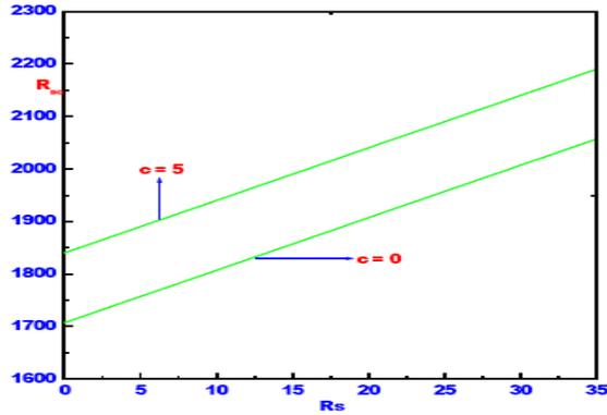
**Figure 11:** Effect of salinity Rayleigh number and viscosity variation  $c$  on critical Rayleigh number with  $L = 0.1$ ,  $R_s = 5 \times 10^3$  for stationary convection.
