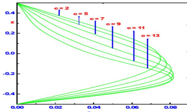
**Figure 10:** Temperature perturbation  $\theta(z)$  for different values of viscosity ratio  $c$  with  $L = 0.1$ ,  $R_s = 5 \times 10^3$  and R/R boundary conditions.
