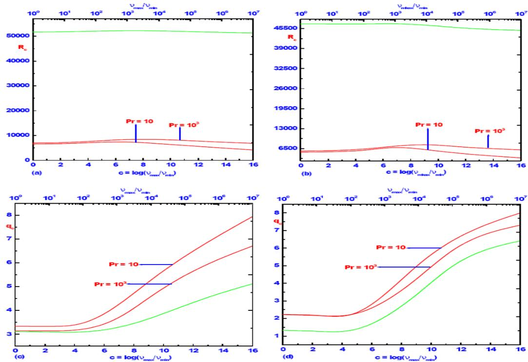
**Figure 7:**  $Pr$  versus critical Rayleigh number and critical wave numbers for  $R_s = 5 \times 10^3$  and  $L = 0.1$ . Figs. (a) and (c) are plotted for  $R/R$  boundaries. Figs. (b) and (d) are plotted for  $F/F$  boundary conditions. Green and red lines are correspond represent stationary and oscillatory convections, respectively.
