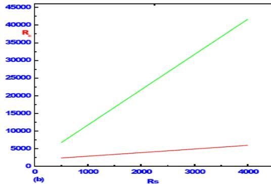
**Figure 12:** Effect of salinity Rayleigh number  $c = 5$  on critical Rayleigh number with  $L = 0.1$ ,  $R_s = 5 \times 10^3$ ,  $P_r = 10^3$ . Green line corresponding to stationary convection and red line corresponds to oscillatory convection.
