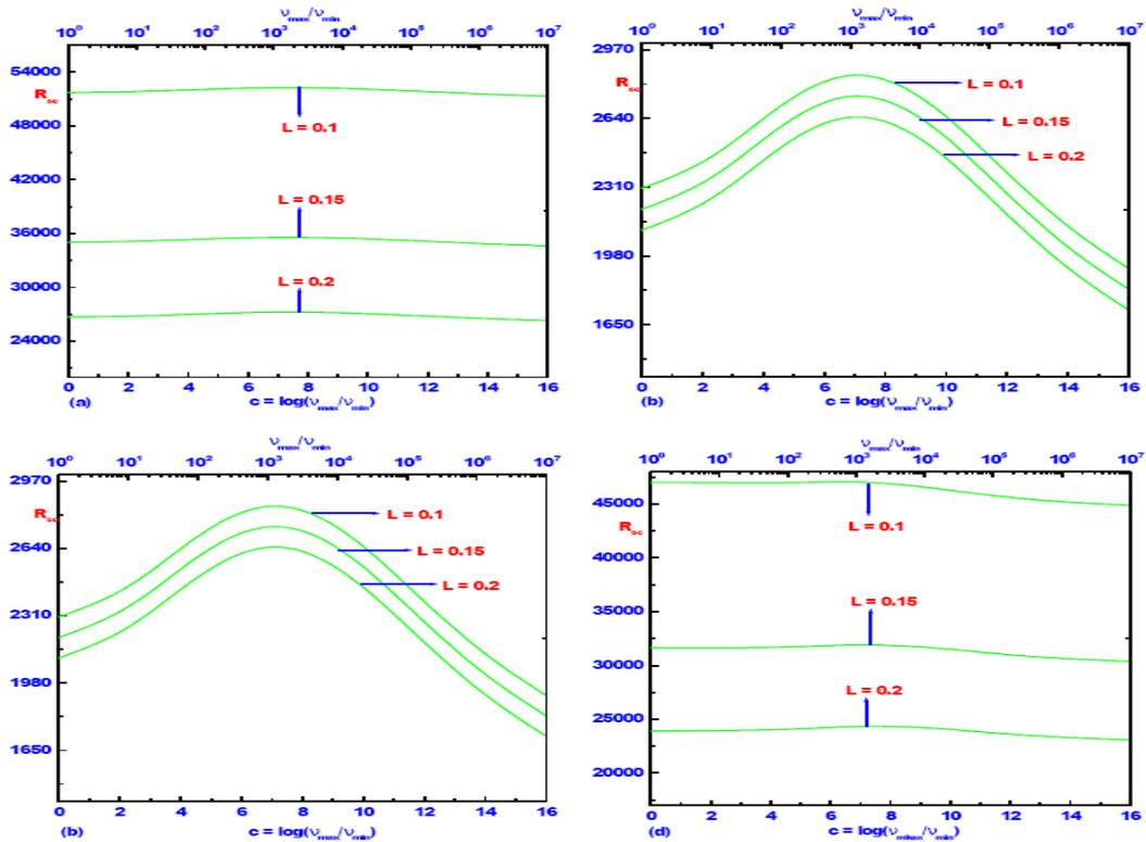
**Figure 3:**The effect of Lewis number  $L$  and viscosity ratio  $c$  on  $R_{sc}$  for  $R_s = 5 \times 10^3$ . Numerically plotted neutral stability curves to represent onset of stationary convection for exponential fluid. Figure 3(a-d) are plotted for  $R/R$ ,  $R/F$ ,  $F/R$  and  $F/F$  boundary conditions respectively.
