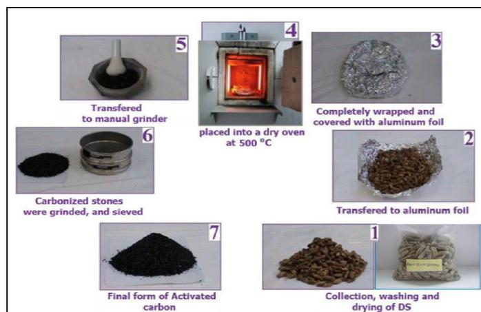
**Figure 9.** The production process of AC from date stones[86]
