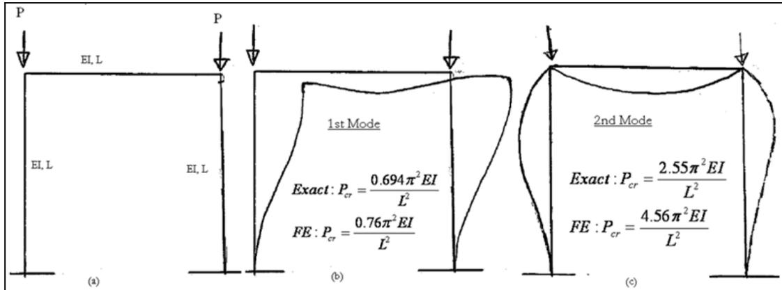
Figure 1: (a) Portal frame; (b) 1<sup>st</sup> Mode deformed shape; (c) 2<sup>nd</sup> Mode deformed shape
