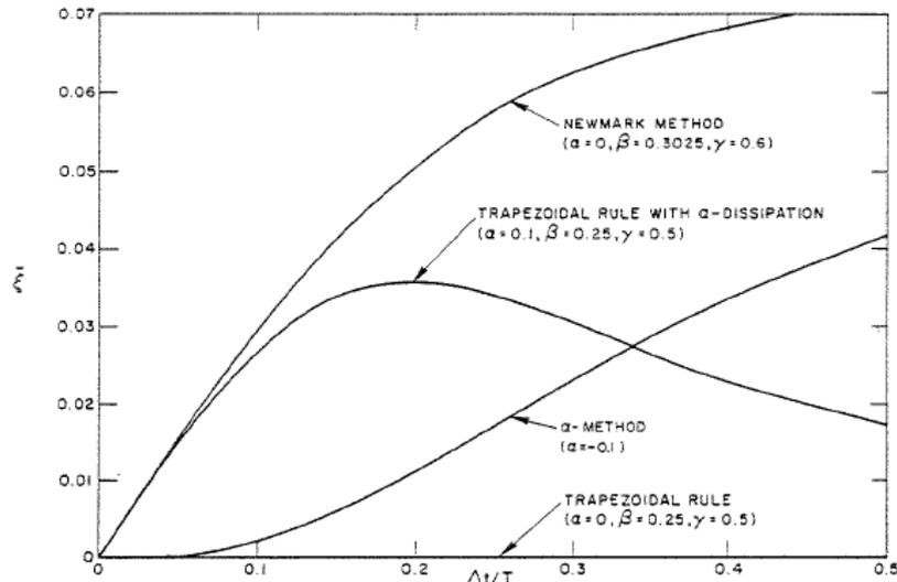
**Figure 3:** Algorithmic damping ratios versus  $\Delta t/T$  for  $\alpha$ -method and some Newmark schemes (adapted from Hilber, 1976 [1])
