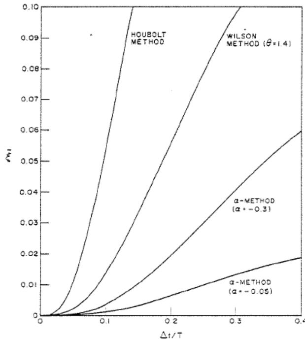
**Figure 4:** Algorithmic damping ratios versus  $\Delta t/T$  for  $\alpha$ -method and Houbolt and Wilson schemes (adapted from Hilber, 1976 [1])
