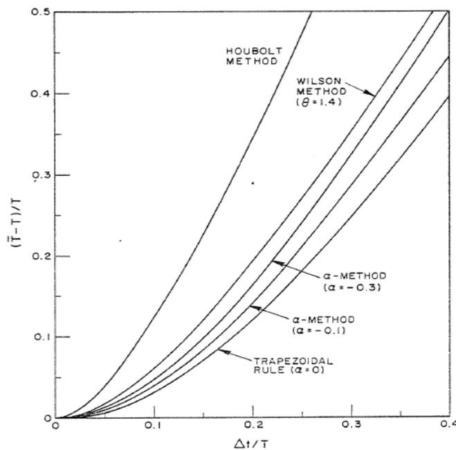
Figure 6: Relative period error versus  $\Delta t/T$  for different algorithms (adapted from Hilber, 1976 [1])
