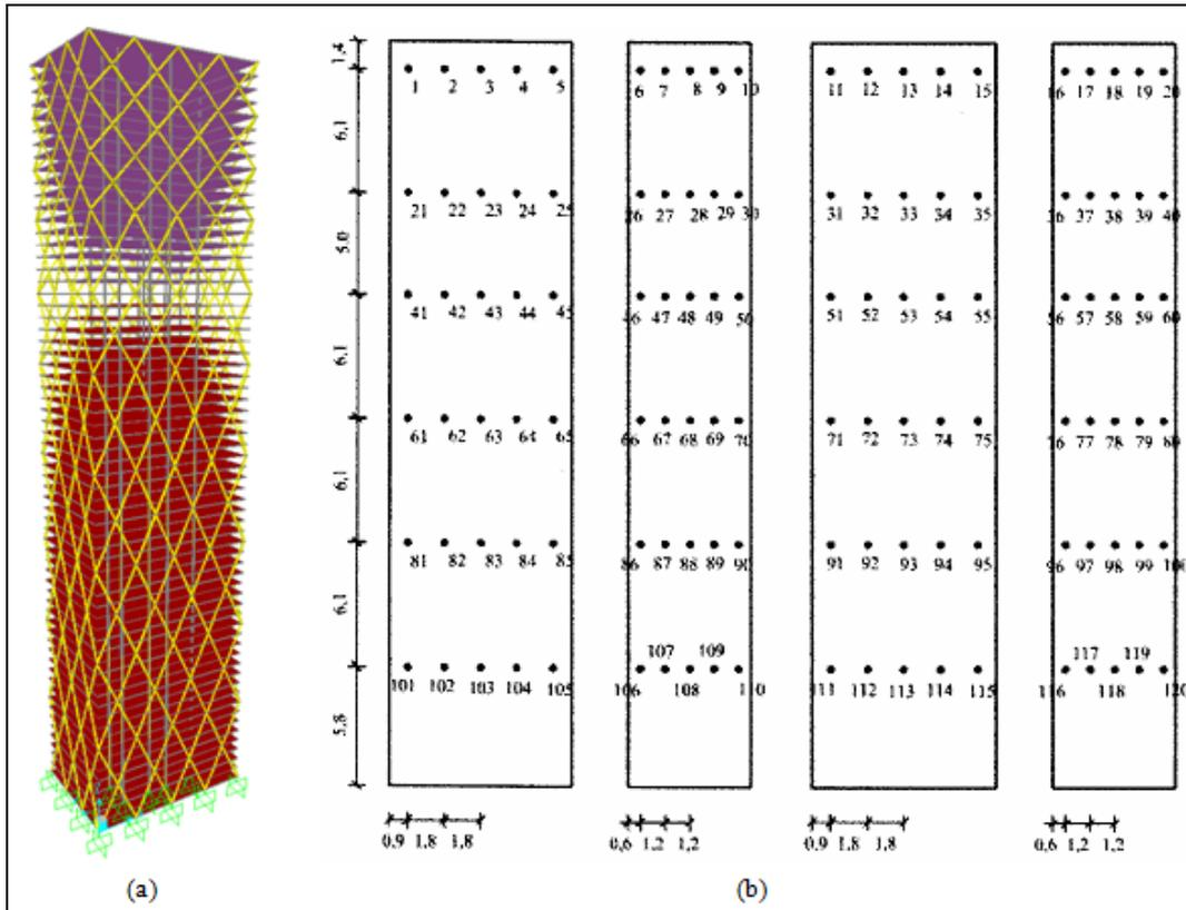
Figure 7: (a) 3-D view of 64-story Diagrid structure; (b) Tap location around the building faces for BLWT (adapted from NIST & CRIACIV, Prato, Italy)
