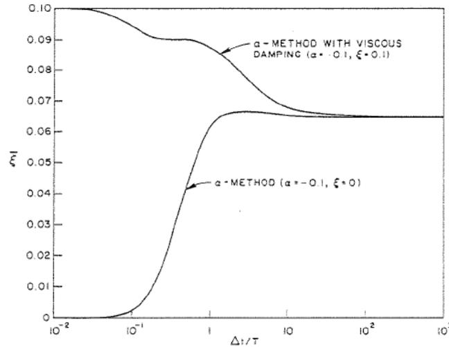
Figure 5:  $\alpha$ -method with and without viscous damping (adapted from Hilber, 1976 [1])
