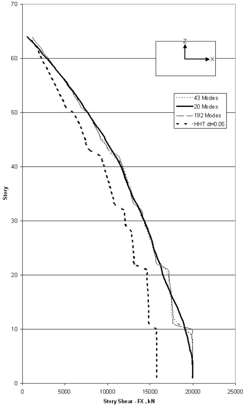
Figure 9: Comparison of different integration method – Story Shear FX
