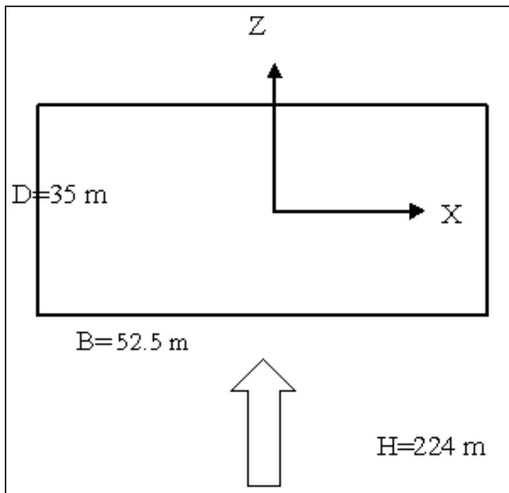
Figure 8: Building Dimensions and Wind Direction
