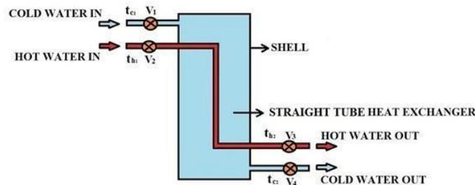
Figure 3: Schematic diagram of the straight tube heat exchanger
