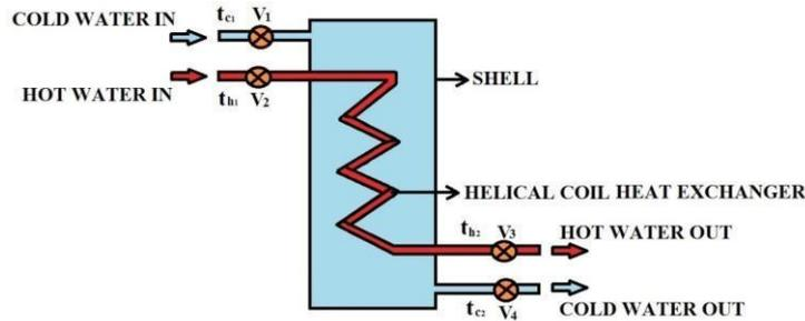
Figure 2: Schematic diagram of the helical coil heat exchanger
