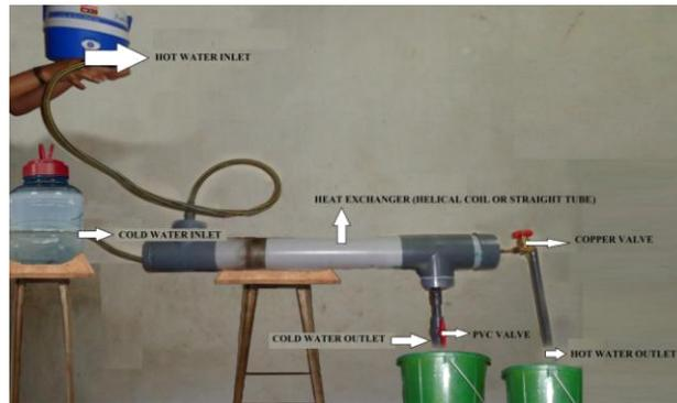
Figure 1: Experimental Test Rig
