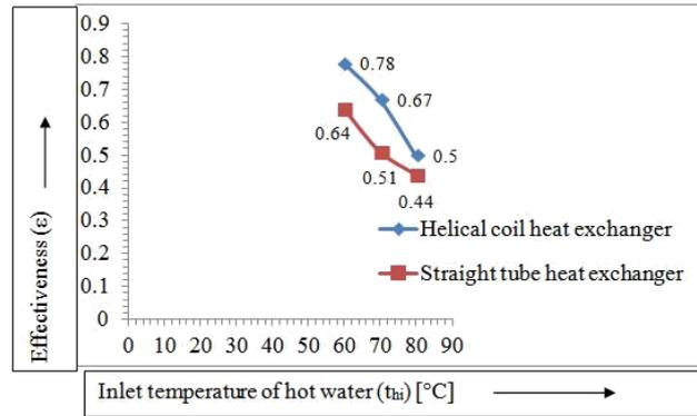
**Figure 4: Variation of effectiveness with inlet temperature of hot water**
