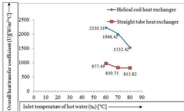
**Figure 5: Variation of overall heat transfer with inlet temperature of hot water**
