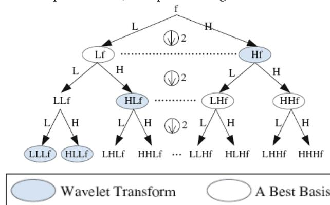
Fig. 1. Illustration of the wavelet packet decomposition.
