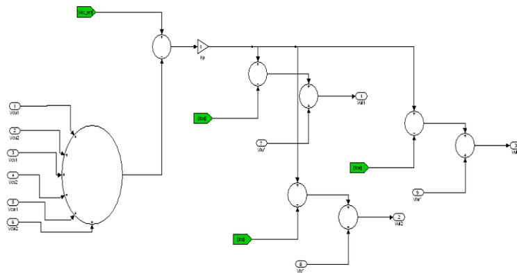
**Fig.5** Block diagram of individual voltage control
