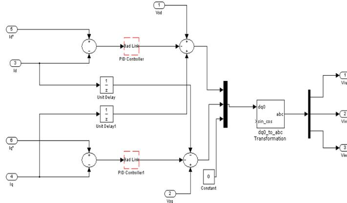
Fig.2 Block diagram of decoupled current control
