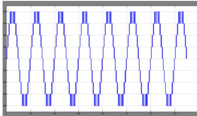
Fig.6 Output voltage of 9 level statcom
