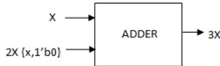
**Fig 2:** Proposed multiplied by 3 Circuit(3MCM)
