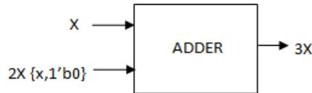
**Fig 2:** Proposed multiplied by 3 Circuit(3MCM)
