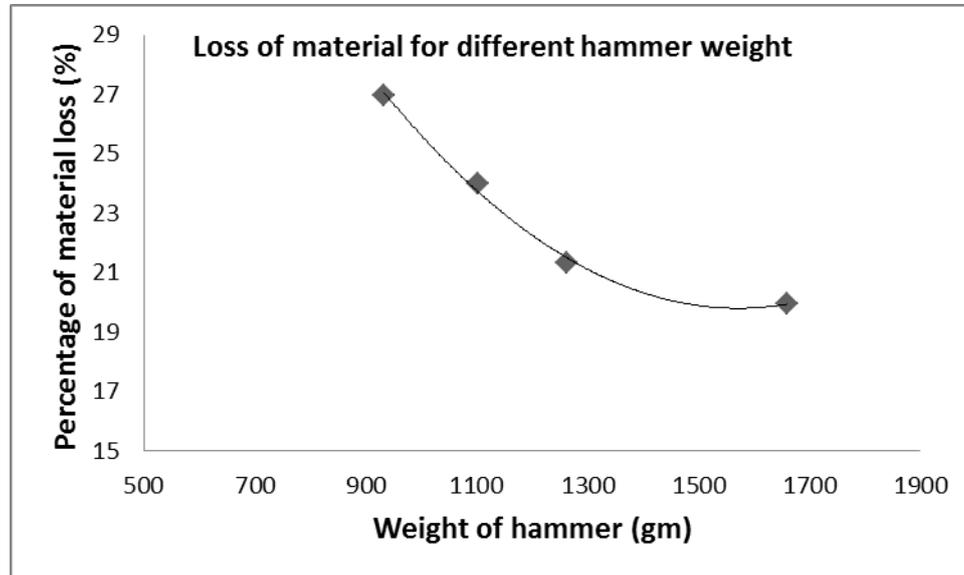
**Fig 5: Loss of material for different hammer weight.**
