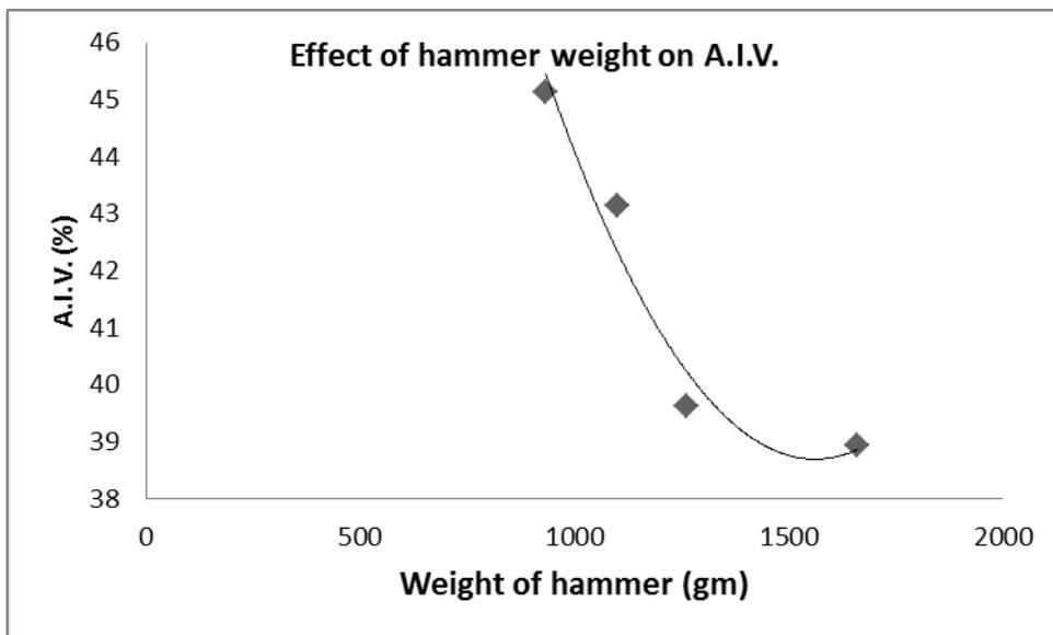
Fig 4: Effect of hammer weight on A.I.V.
