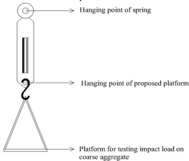
**Fig 2: Experimental arrangement for impact load testing.**
