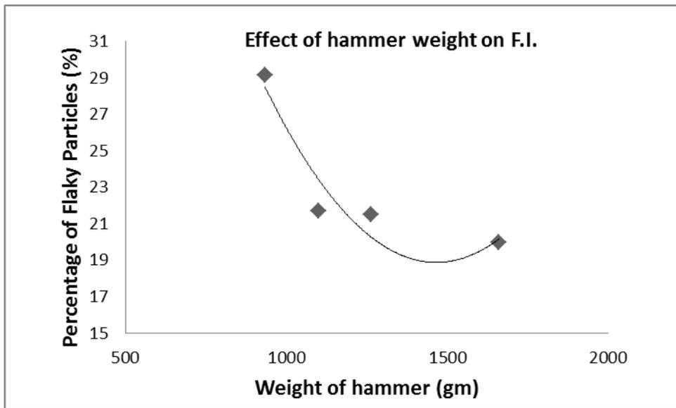
Fig 3: Effect of hammer weight on flaky particles.
