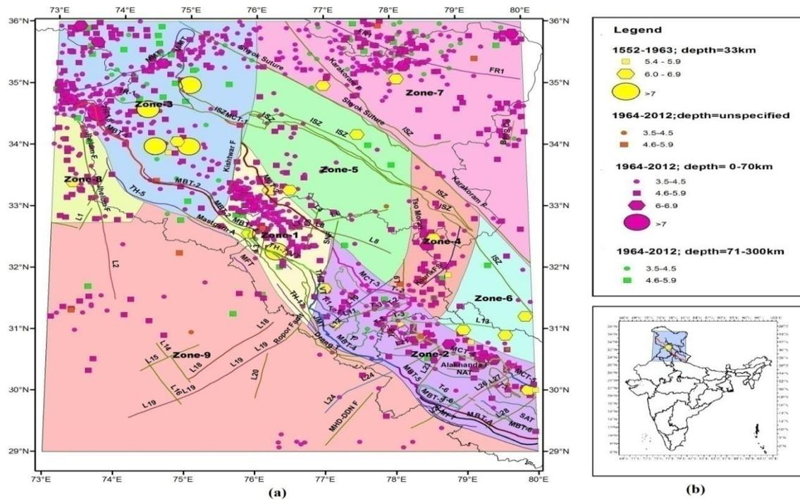
Figure 1. (a) Seismo-tectonics and Seismogenic Source Zones delineated for Himachal Pradesh and contiguous regions, (b) Main Boundary Thrust (MBT), Main Central Thrust (MCT) and epicenter of Kangra earthquake shown on Map of India. Box shows study area.
