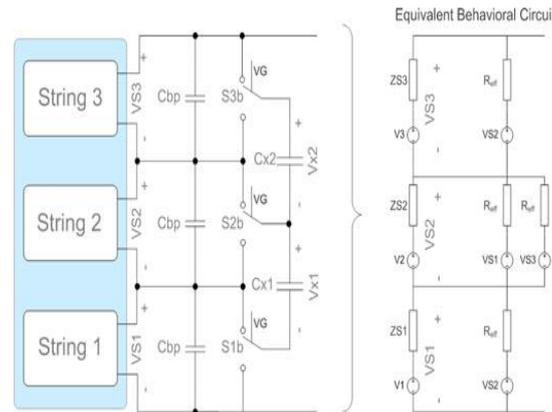
Fig. 5. SC ladder converter for balancing one PV module
