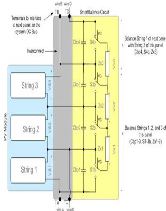
Fig. 8. Distributed converter circuit architecture
