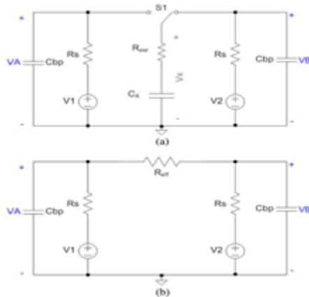
Fig.6. (a) SC conversion cell. (b) Behavioral equivalent
