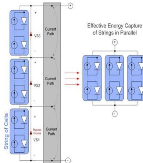
Fig.4. Conversion process forms an effective parallelization of PV strings cells per panel
