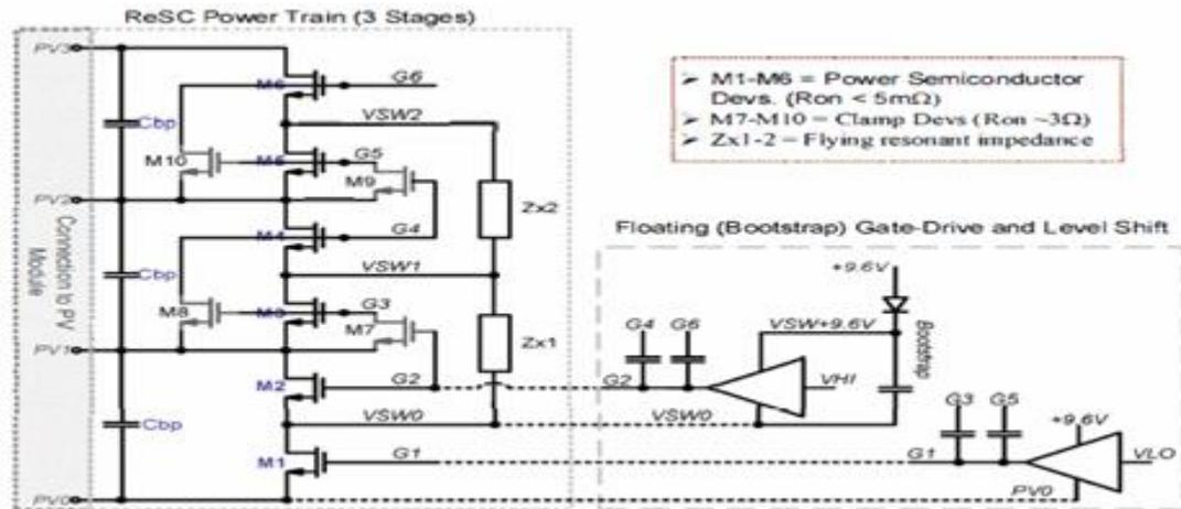
Fig. 9 Floating gate-drive and level - shift circuit for ReSc three stages of the Re-SC power train and configuration with high-voltage gate drivers
