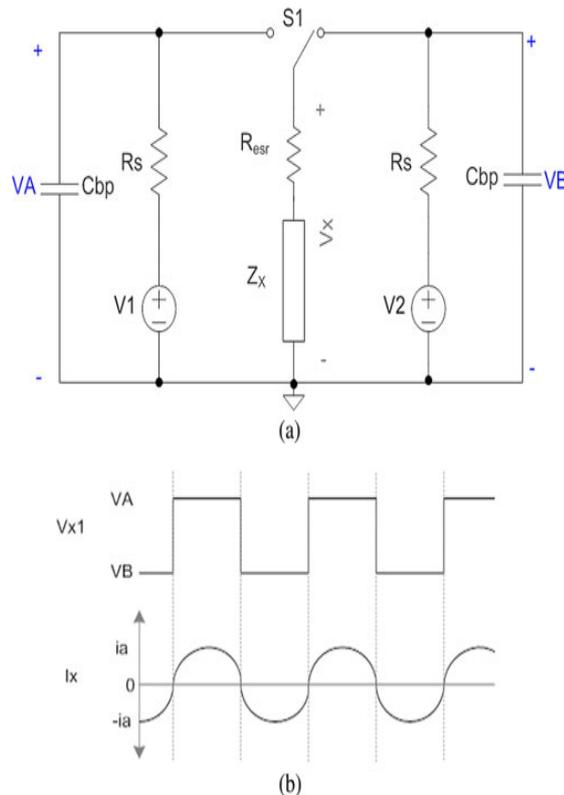
Fig. 7. (a) Resonant impedance conversion cell. (b) Current and voltage waveforms Limitations of the SC
