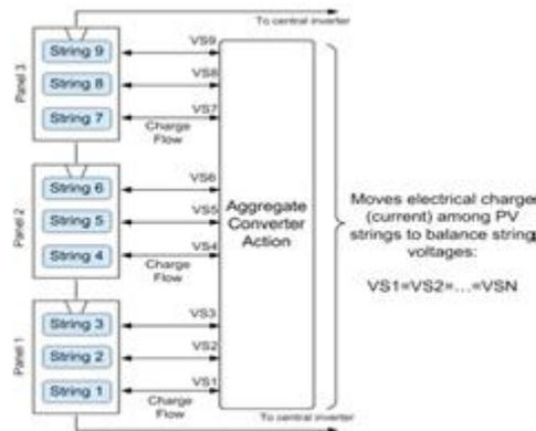
Fig. 2. Proposed resonant ladder converter architecture
