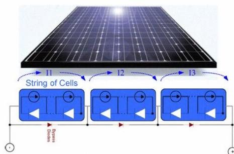
Fig. I. Typical PV module with 3 strings of cells
