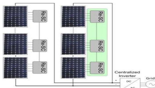
Fig. 3. Effective aggregate converter for one string of PV modules.
