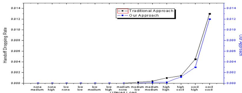
The above fig gives the effect of offered load on handoff dropping rate. In the above fig the proposed method gives best result than the traditional approach even offered load varies. Our proposed model reduces the hand off dropping rate by up to 0.480%.
