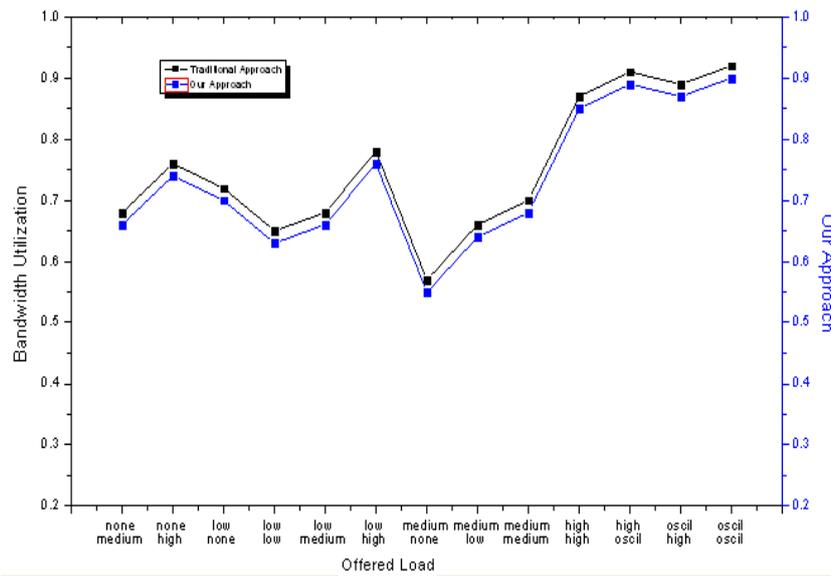
In the above fig, our proposed approach shows better result than the traditional approach on overall bandwidth utilization even if offered load varies. In the above graph we considered bandwidth utilization on y axis and load on x axis. This proposed method increases bandwidth utilization by 2.5% as compared with traditional approach.
