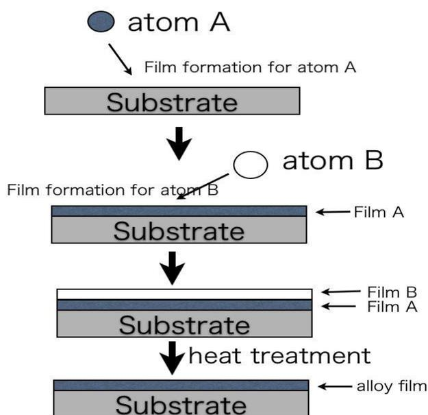
Fig.8 Concept for Heating Stacked Single Layers Process
