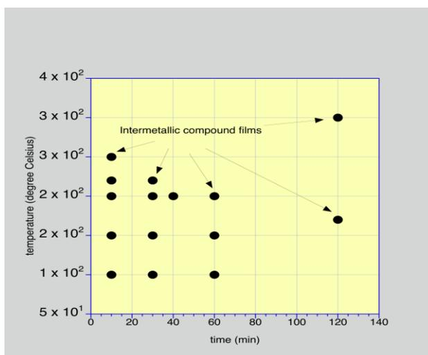
Fig.9 Heat Treatment Conditions and Produced Film
