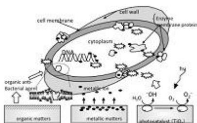
Fig.2 Mechanism of antibacterial effects for various materials.
