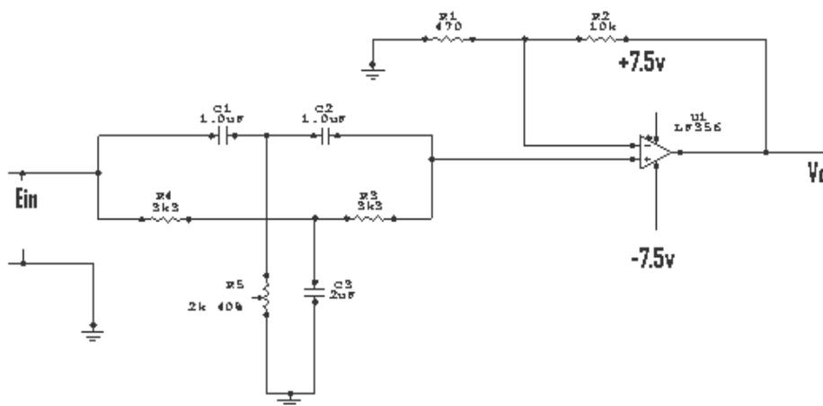
FIG: 4 THE CIRCUIT DIAGRAM OF THE TWIN-T FILTER
