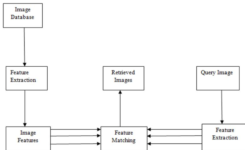
Figure 1. Block diagram of Content based image retrieval
