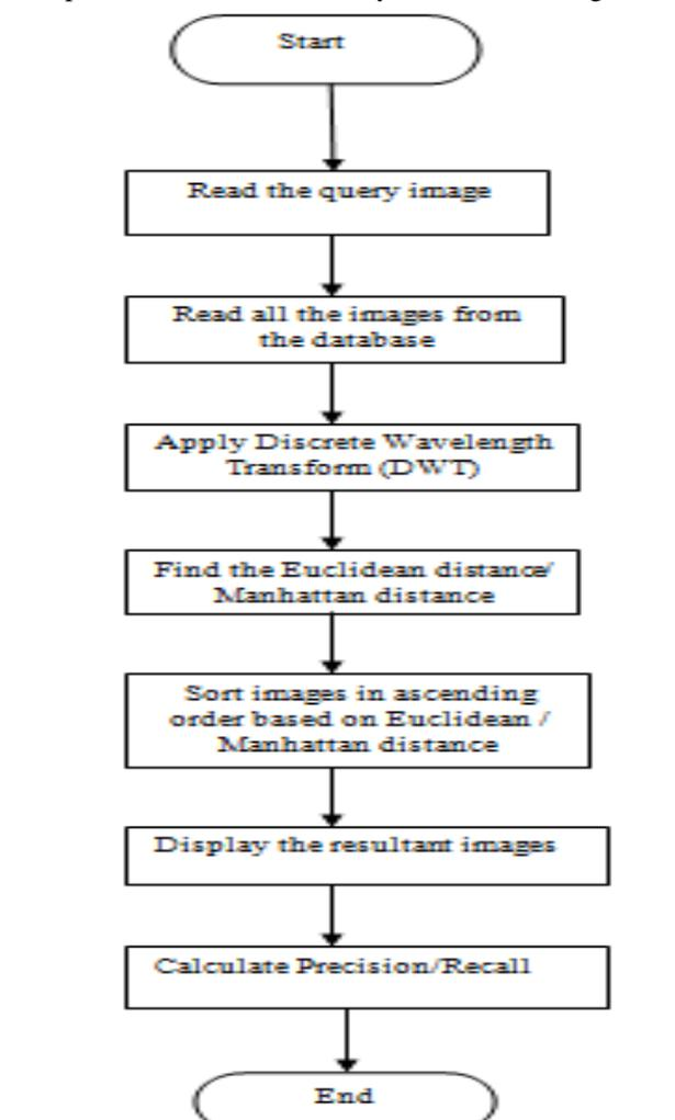
Figure 3 Flow chart of image retrieval without using CLAHE
