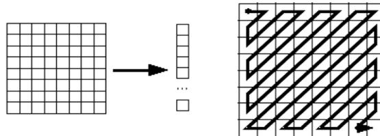
Fig 2: Zigzag scanning
