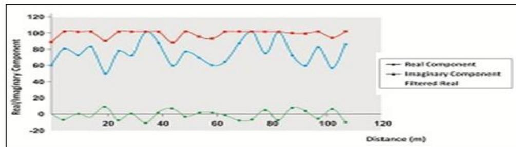
**Fig 5: Electromagnetic (VLF) Conductivity Profile along traverse3, E-W direction at 5m interval**
