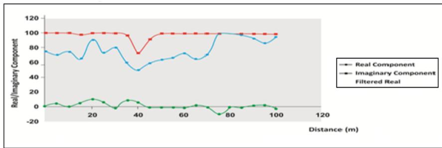
**Fig1: Electromagnetic (VLF) Conductivity Profile along traverse1, S-N direction at 5m interval**
