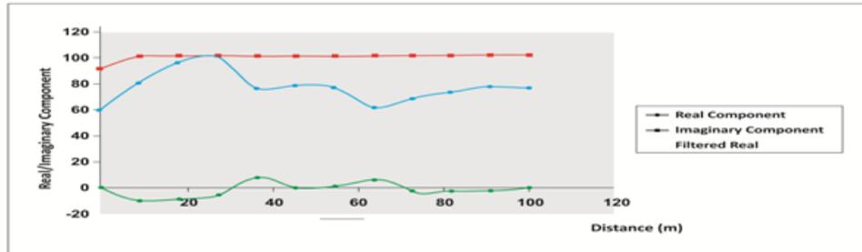
**Fig 6: Electromagnetic (VLF) Conductivity Profile along traverse3, E-W direction at 10m interval**
