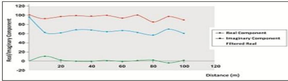
**Fig 4: Electromagnetic (VLF) Conductivity Profile along traverse2, E-W direction at 10m interval**
