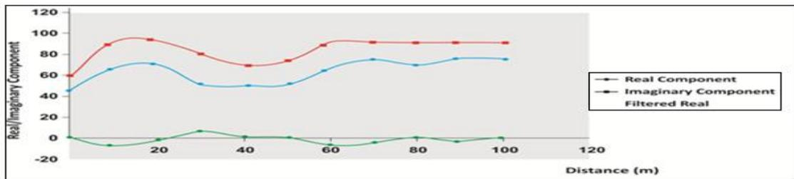
**Fig 2: Electromagnetic (VLF) Conductivity Profile along traverse1, S-N direction at 10m interval**
