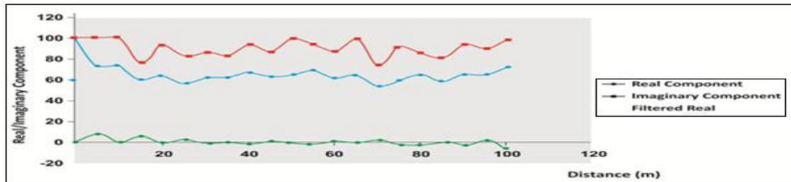
**Fig 3: Electromagnetic (VLF) Conductivity Profile along traverse2, E-W direction at 5m interval**
