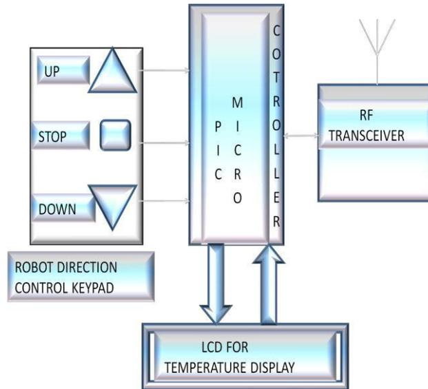
**Fig. 5:** Direction controller Handset Block diagram
