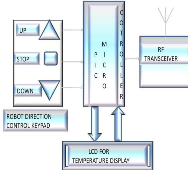
**Fig. 5:** Direction controller Handset Block diagram
