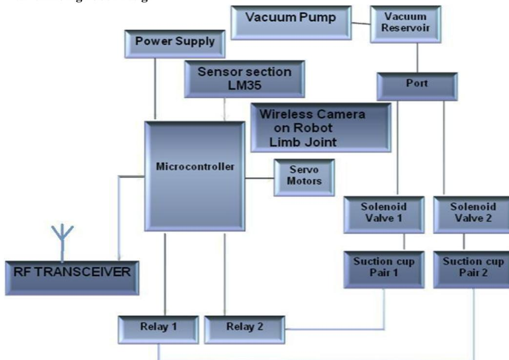
Fig.4 : Total Block diagram
