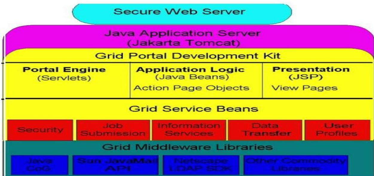
Figure 1.2: GPDK architecture, with the grid service beans and grid middleware libraries shown
