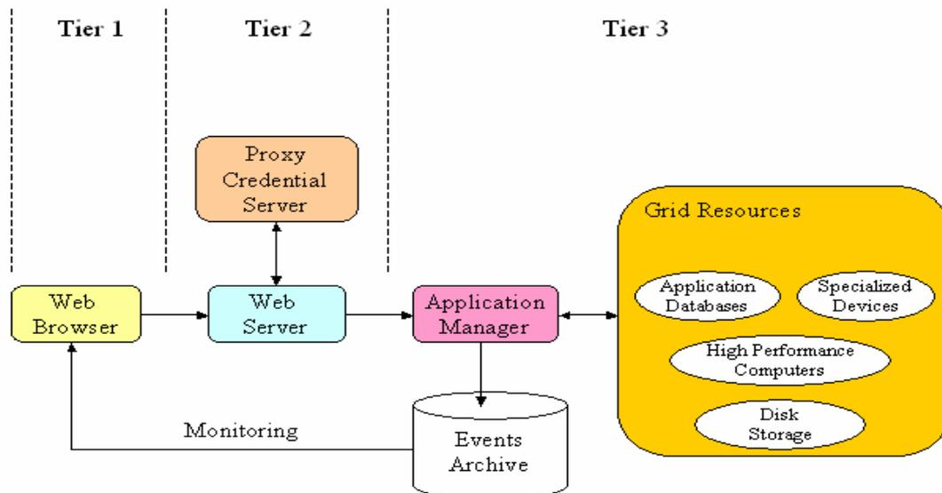
Figure 1.1: First Generation Portal architecture, with its three-tiers
