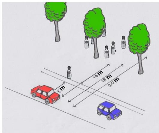
Figure 3: Sketch of the Position of SLM Placement Relative to Highway
