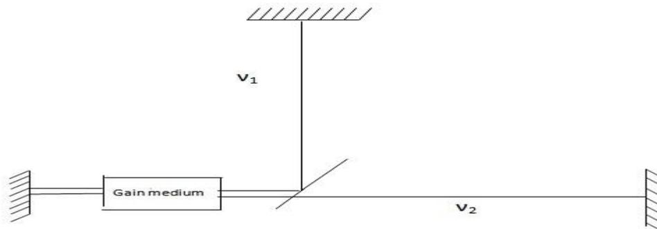
Fig.2 (b) Doubly Resonant Cavity
