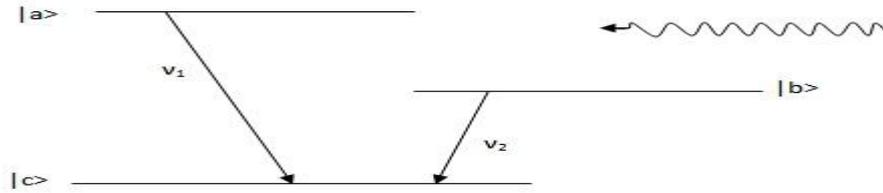
Fig 5. In the three level atoms, the two upper levels  $|a\rangle$  and  $|b\rangle$  are coupled via a strong microwave frequency  $\nu_3$ . The emissions from the  $(|a\rangle \rightarrow |c\rangle)$  and  $(|b\rangle \rightarrow |c\rangle)$  transitions are strongly correlated.
