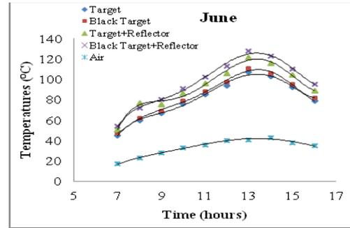
Fig. 6, Various target temperatures variations with time on June
