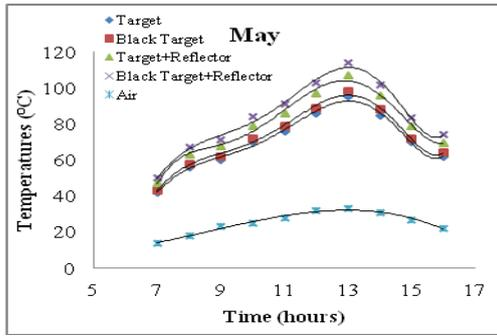
Fig. 5, Various target temperatures variations with time on May
