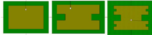
Fig. 1: The Antenna Structures 1(a) Basic Square (b) First Iteration Fractal (c) Second Iteration Fractal.
