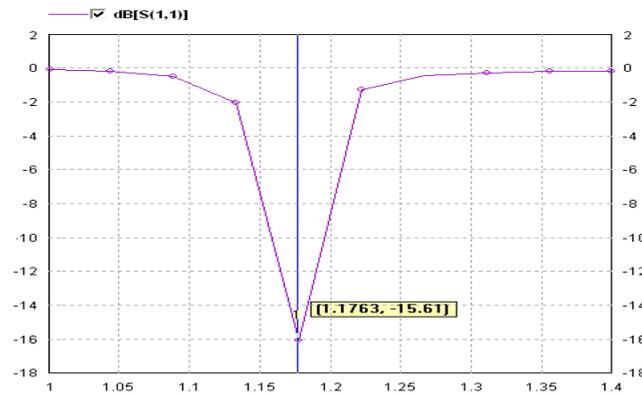
Fig. 5: S-Parameter Display of second Iteration Fractal Patch at 1.776GHz
