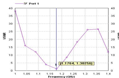
Fig. 8: VSWR of Stacked Fractal Patch Antenna
