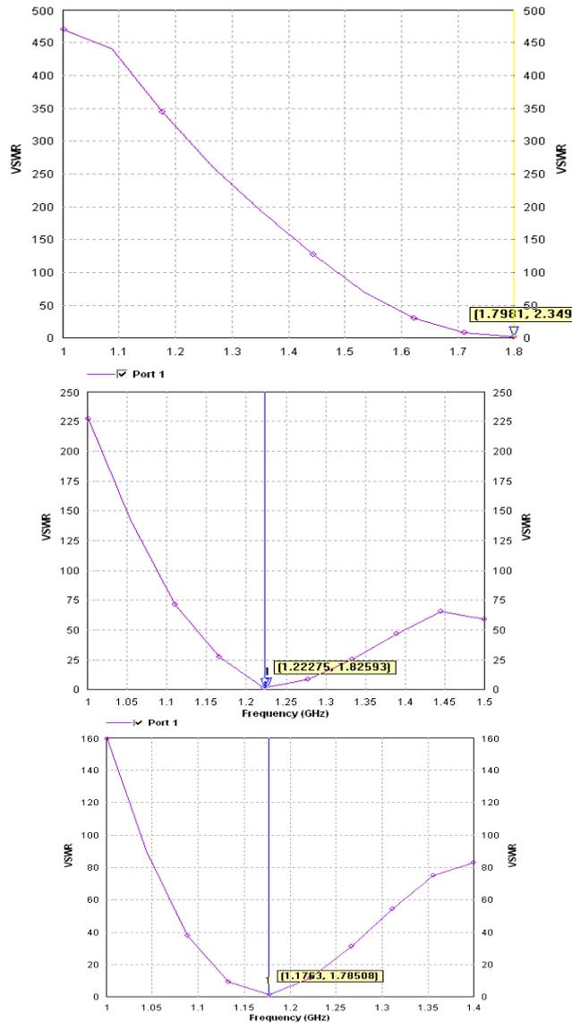
Fig. 7: VSWR of Antenna Structures 1 at Frequencies 1.8, 1.227, 1.776GHz
