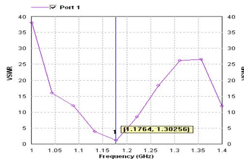
Fig. 8: VSWR of Stacked Fractal Patch Antenna
