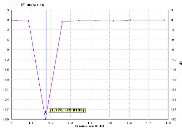
Fig. 6: S-Parameter Display of Stacked Fractal Patch Antenna 2
