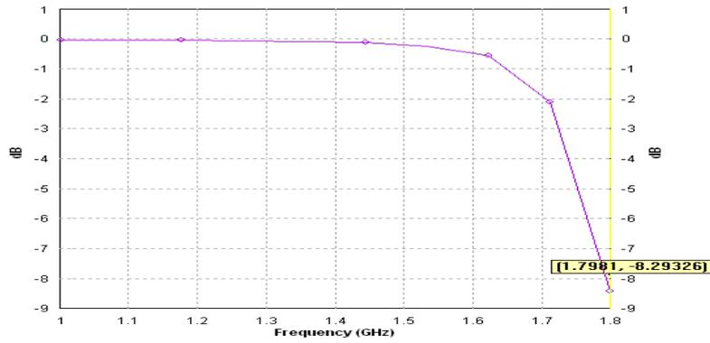
Fig. 3: S-Parameter Display of Basic Patch Antenna at 1.8GHz
