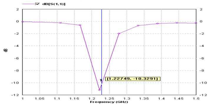
Fig. 4: S-Parameter Display of First Iteration Fractal Patch at 1.227GHz
