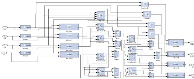
Fig 5. Check node design in Simulink
