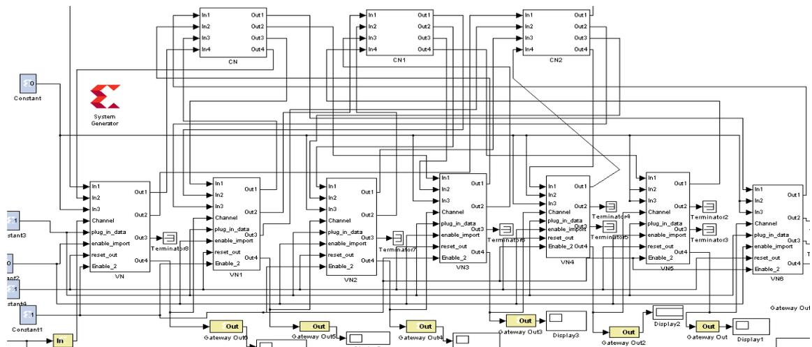
Fig 6. LDPC Decoder design in Simulink
