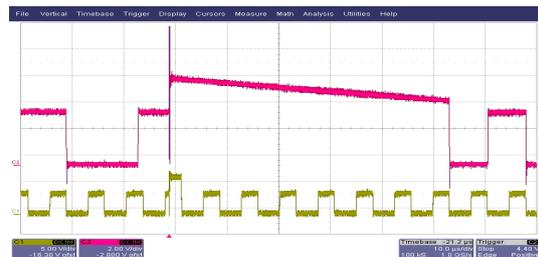
Fig. 6 Output when data and clock are triggered at a high
