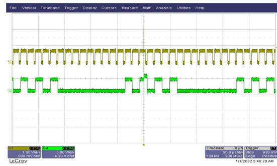
Fig. 22 Output for 0.047µf coupling capacitor
