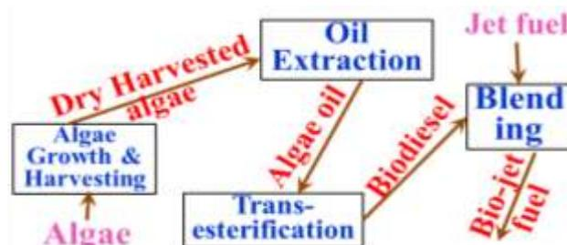
Figure 2: Bio-jet fuel production by the blending process
