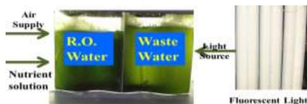
Figure 3: Experimental setup for microalgae growth.
