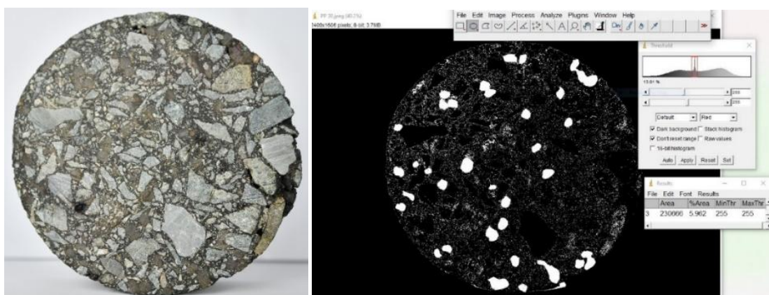
Figure 16 Results of image analysis of AC-WC cross-section with 30% PP substitution
