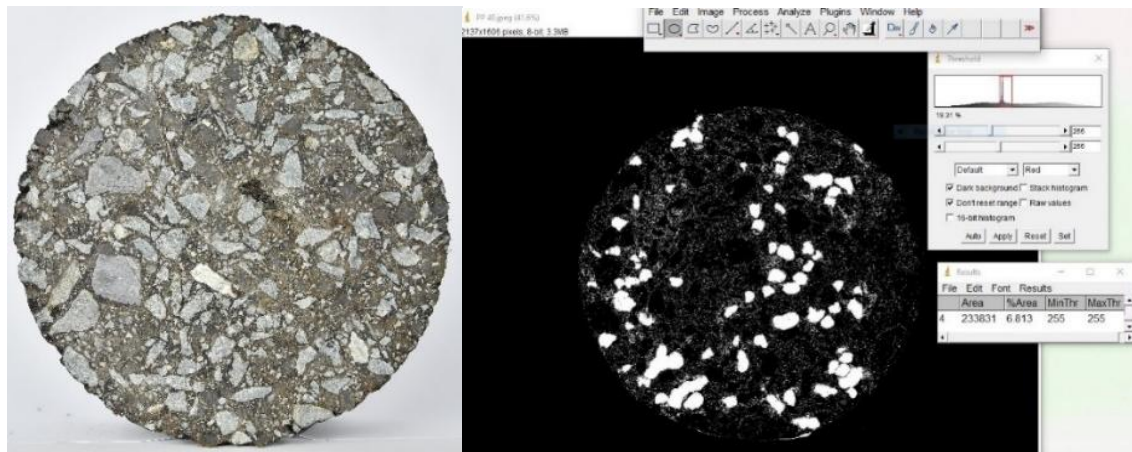
Figure 17 Results of image analysis of AC-WC cross-section with 40% PP substitution
