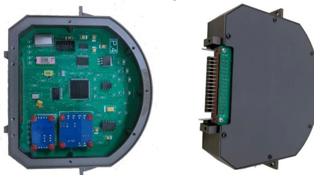
Figure 6. Image of electronic panel of the command decoding block
