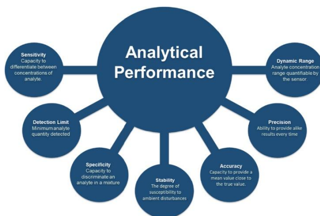
Figure 3: Analytical parameters for validation of biosensor performance (Ana I. Barbosa et al., 2020)
