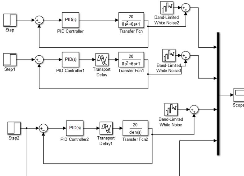
As shown in Figure 14, the transfer function is controlled by a PID controller. There are four blocks in this diagram: the PID module, the step function, the Band limited white Gaussian noise, the transfer function, and the scope for displaying the results. Fuzzy logic controller with band-limited white Gaussian noise is shown in figure 15, along with the step signal, transfer function, and output scope.
