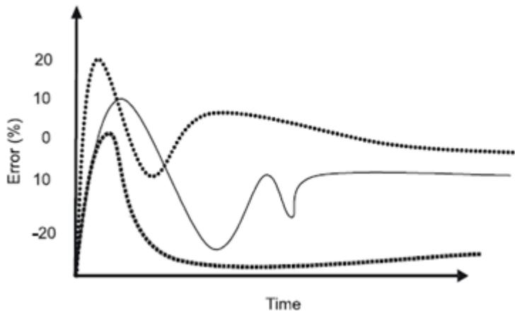
Figure 3: Cycling in PID Controller
