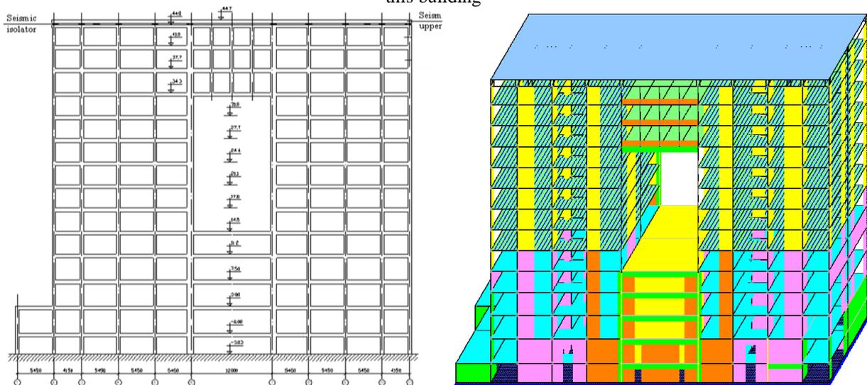
**Figure 2.** Vertical structural elevation of the building, the seismic resistance of which was suggested to be increased by the seismic isolated upper slab method (proposed by the author of this paper), and the design model of this building
