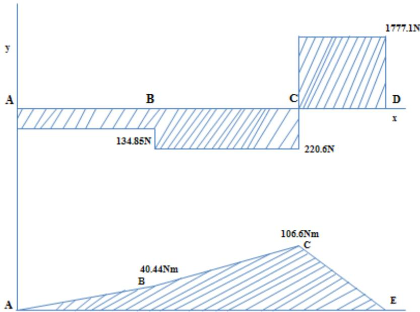
Figure 3; Shearing and bending moment diagrams of the shaft.
