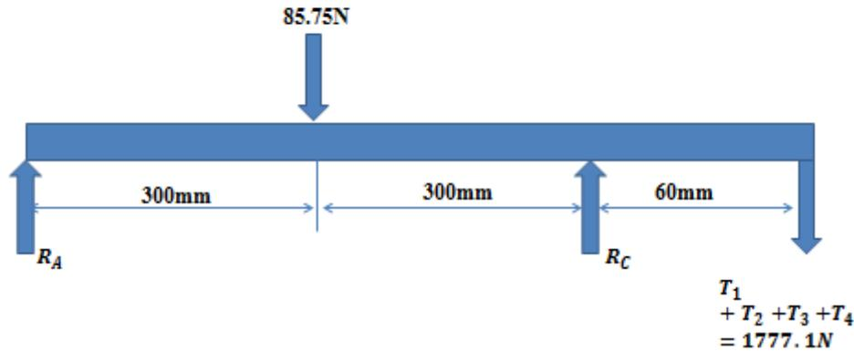
Figure 2; Analysis of forces on cylinder shaft.
