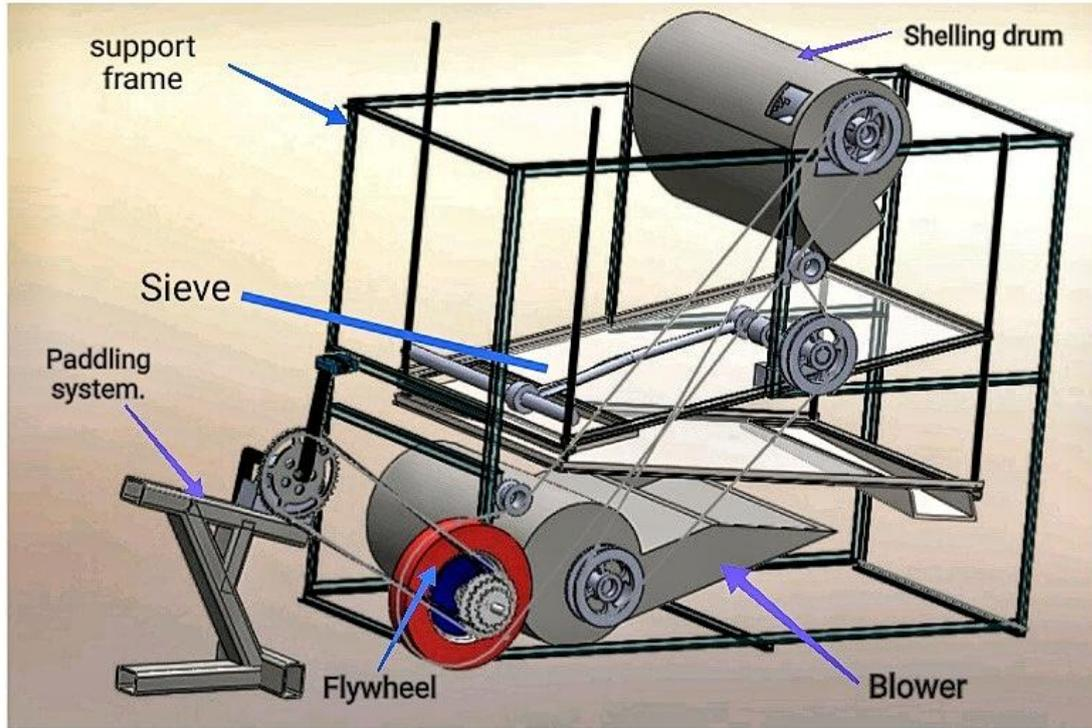
Figure 1. Schematic diagram of the prototype machine.
