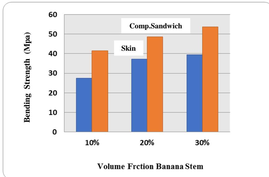
This is due to the increasing number of fibers that will contribute very well in bearing the load, so that the load given to the composite will be held by the fiber to the maximum load limit which causes the composite
