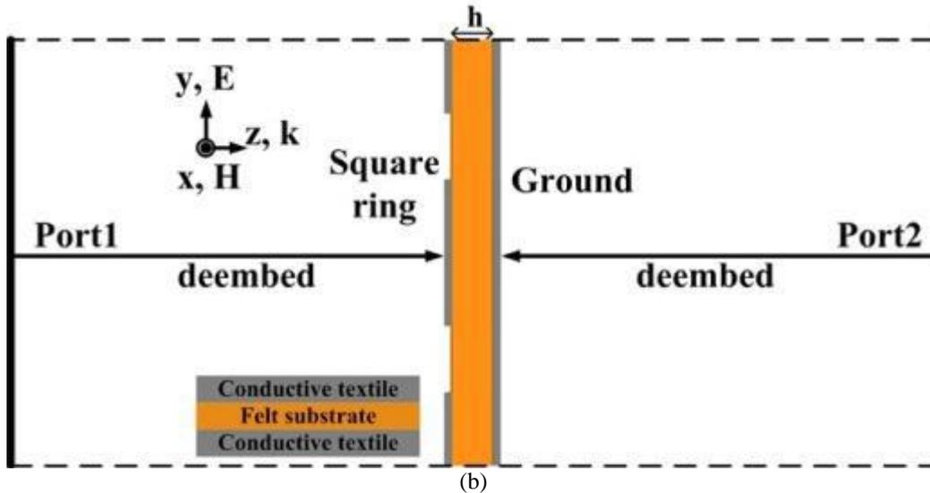
**Fig. 1.** Geometry of the proposed WMMA ( $a = 30$  mm,  $b = 9.7$  mm,  $w = 2$  mm,  $g = 5$  mm, and  $h = 1$  mm): (a) magnified view of the unit cell and periodic structure, and the (b) side view indicating the direction of the incident waves.
