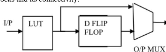
Fig. 1 Basic Logic element
