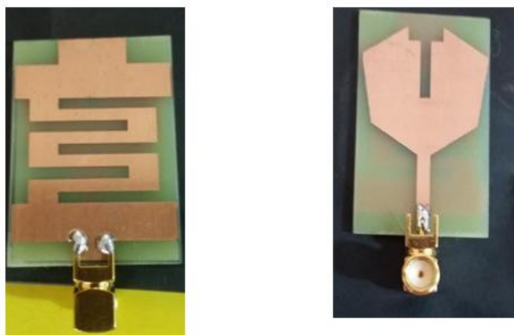
Fig 10: Fabricated Front and Rear view of Antenna
