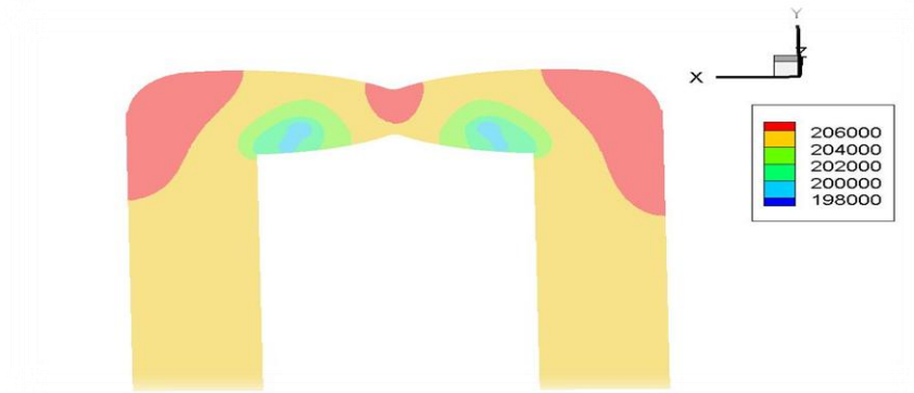
Fig. 6 Distribution of static pressure on a cross-section at X-Y plane
