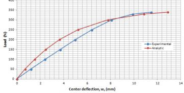
Fig.5: variation of the center deflection  $w_c$  according to the load P of the test specimen E.
