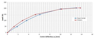
**Fig.6** variation of the center deflection  $w_c$  according to the load P of the test specimen F.
