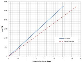
Fig 4: variation of the center deflection  $w_c$  according to the load P of the test specimen A
