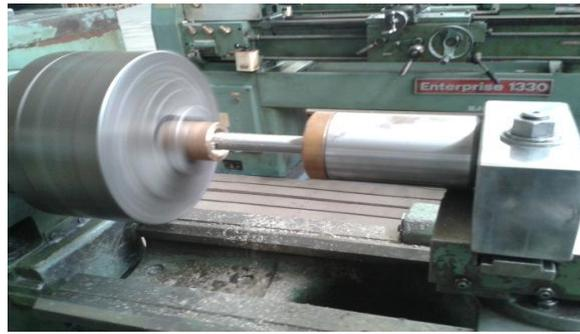
**Figure 4** MRF Boring Bar installed on Lathe
