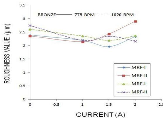
**Figure 12** Surface roughness v/s input current
