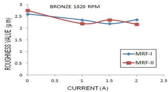
**Figure 11** Surface roughness v/s input current at 1020 RPM
