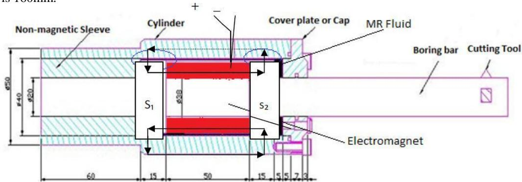
**Figure 1** Diagram of Magneto-rheological Fluid Boring Bar
