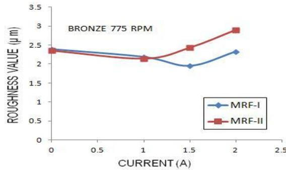
**Figure 10** Surface roughness v/s input current at 775 RPM
