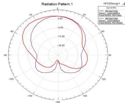
Fig 1(c) Gain radiation pattern of CPW fed Rectangular Patch Antenna
