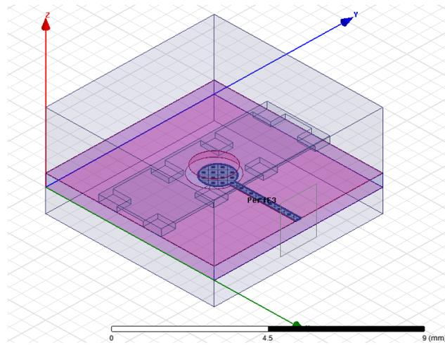
Fig. 2(a) Simulation model of CPW-fed Circular Patch Antenna
