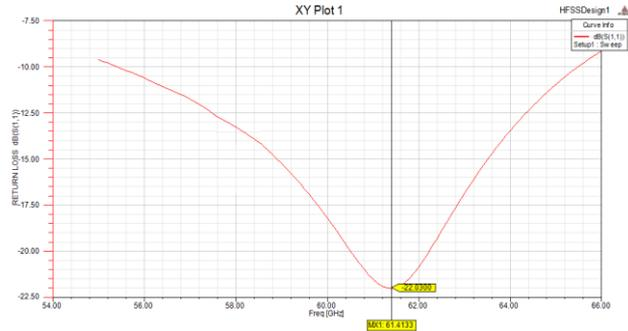
Fig. 1(b) Return loss plot of CPW fed Rectangular Patch Antenna
