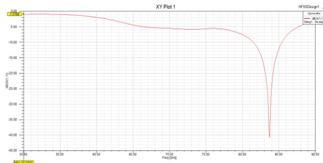
Fig. 3(b) Return loss plot of CPW-fed patch antenna with Inductive coupling
