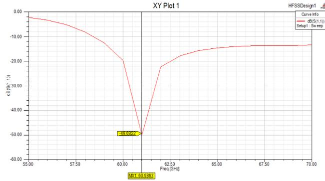
Fig. 4(b) Return loss plot of CPW-fed patch antenna with capacitive coupling
