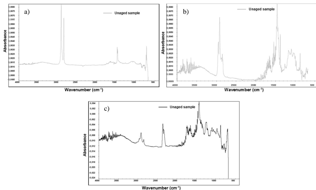
Fig. 7 FT-IR spectra at initial state of: a) HDPE, b) PP, and c) PVC
