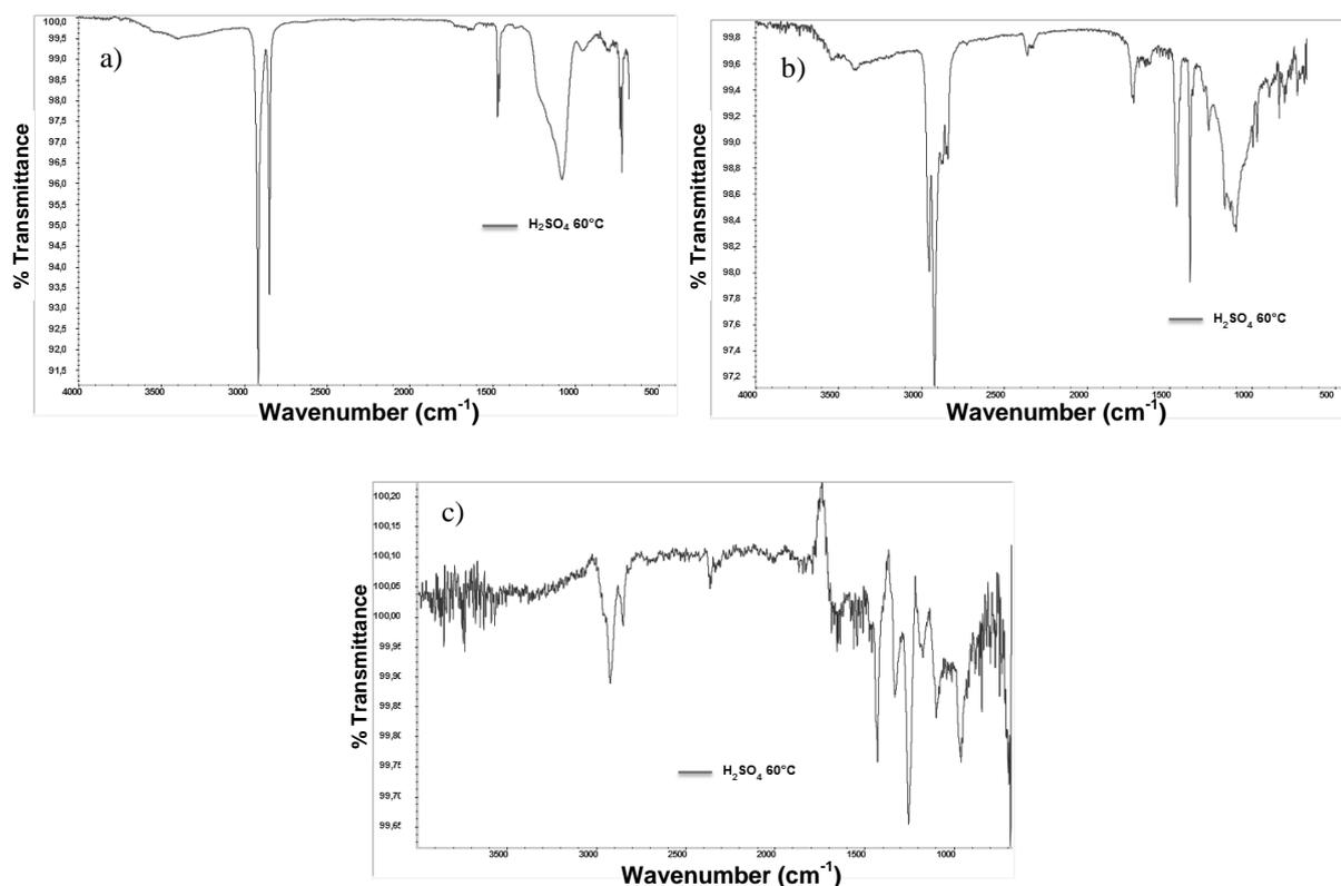
Fig. 8 FT-IR spectra at degraded state of: a) HDPE, b) PP, and c) PVC
