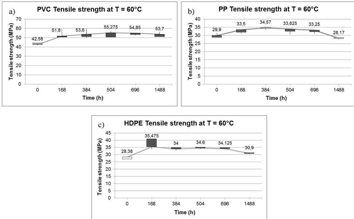
Fig. 5 Tensile strength as function of time for: a) PVC, b) PP and c) HDPE, pipe samples aging in sulfuric acid solution at 60°C
