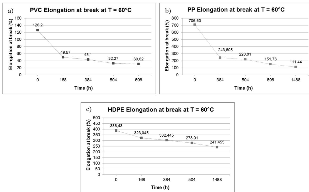
Fig. 6 Elongation at break as function of time for: a) PVC, b) PP and c) HDPE, pipe samples aging in sulfuric acid solution at 60°C
