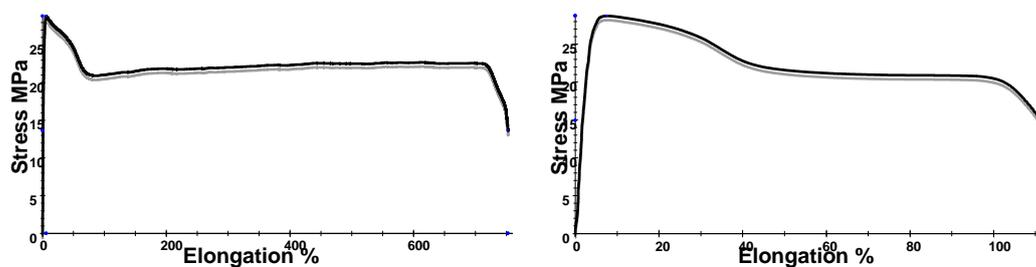
Fig. 3 Curves stress/elongation for PP before and after aging in  $H_2SO_4$  at  $60^\circ C$
