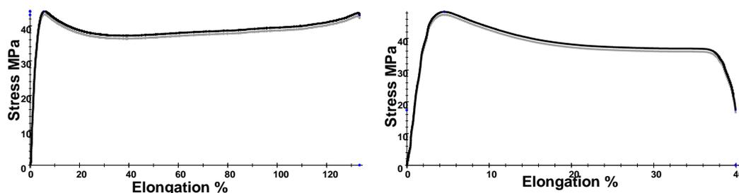
Fig. 4 Curves stress/elongation for PVC before and after aging in  $H_2SO_4$  at  $60^\circ C$
