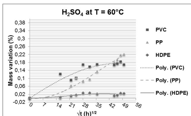
Fig. 1 Weight change as a function of time ( $\sqrt{t}$  ( $h^{1/2}$ )) for PVC, PP and HDPE exposed to  $H_2SO_4$  at  $60^\circ C$
