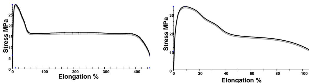
Fig. 2 Curves stress/elongation for HDPE before and after aging in  $H_2SO_4$  at  $60^\circ C$
