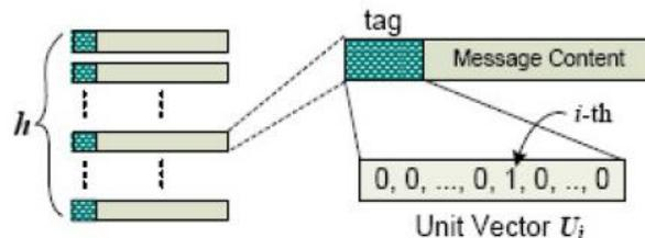
Fig. 5. Packet tagging before source encoding.
