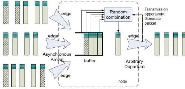
Fig. 2. Random coding (mixing) at intermediate nodes.
