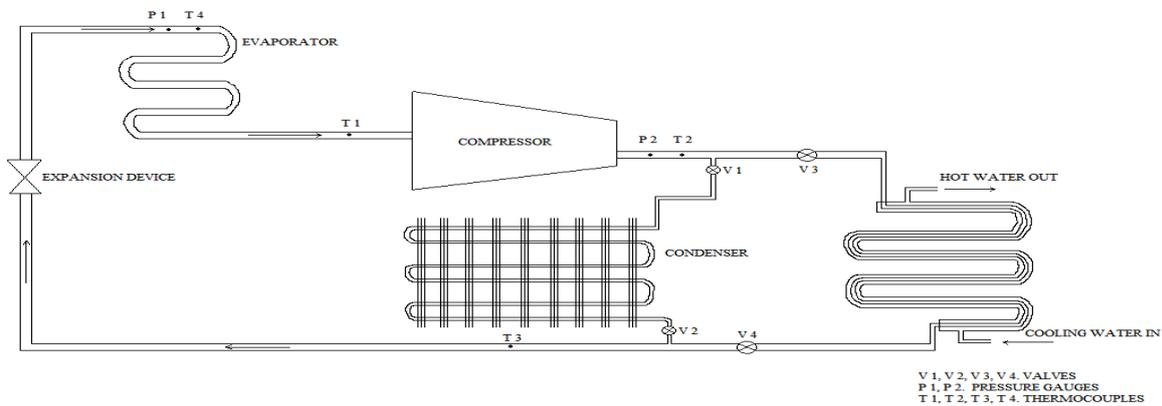
**Figure 2: Schematic diagram of the experimental apparatus**
