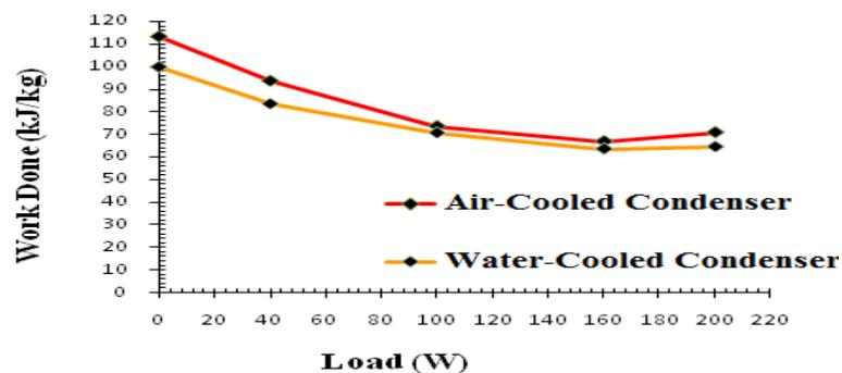
**Figure 3: Variation of work done with load**
