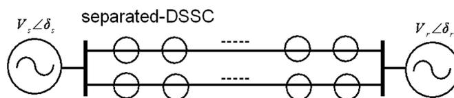
**Fig. 1.** compensation by separated-DSSC modules
