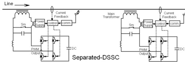
Fig. 3. circuit schematic of separated-DSSC module
