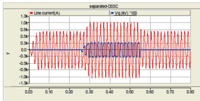
**Fig. 7.** The current in one phase and the injected voltage  $V_q$  by the separated-DSSC module
