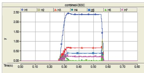
Fig. 10. harmonics of the injected voltage by combined-DSSC
