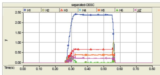
**Fig. 9.** harmonics of the injected voltage by separated-DSSC
