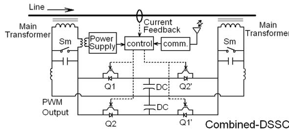
Fig. 4. circuit schematic of combined-DSSC module
