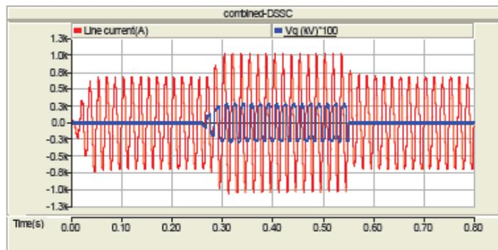
**Fig. 8.** The current in one phase and the injected voltage  $V_q$  by the combined-DSSC module
