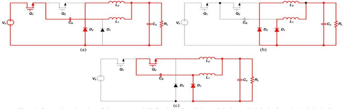
Fig. 4. Operating circuits of the proposed IBC when  $D \leq 0.5$ . (a) Mode 1. (b) Mode 2 or 4. (c) Mode 3.
