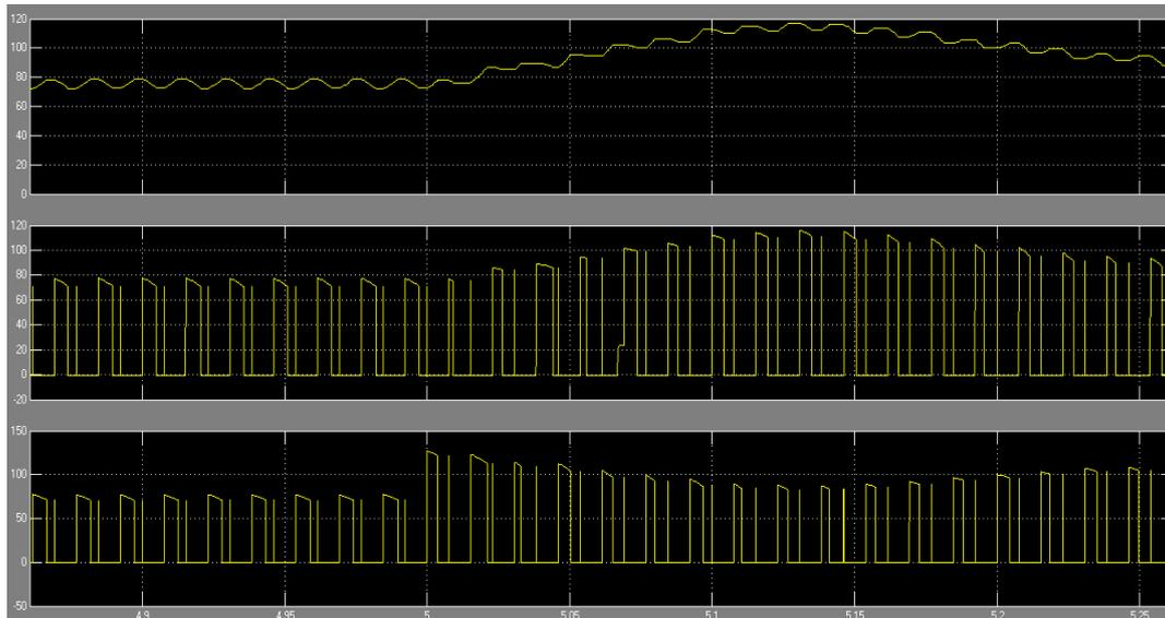
Fig(10). Coupling capacitor voltage wave & Diode 1 voltage& Diode 2 voltage output waveforms For R-Load
