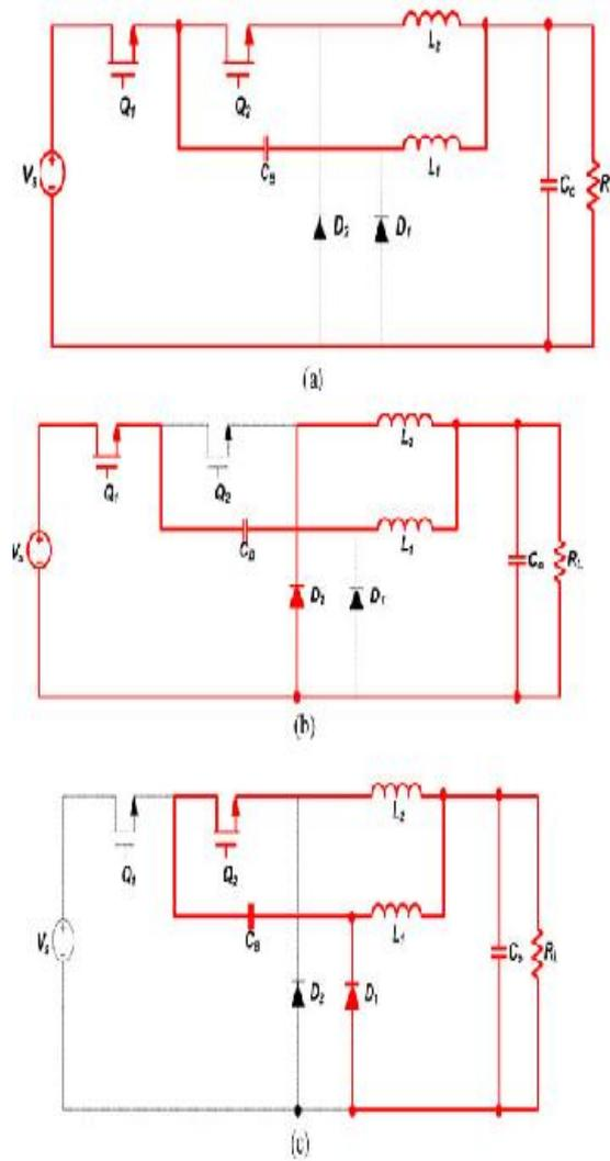
Fig. 5. Operating circuits of the proposed IBC when  $D > 0.5$  (a) Mode1 or 3.(b)Mode2.(c) Mode4.
