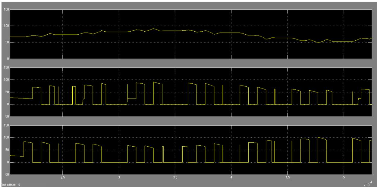
**Fig(13). Coupling capacitor voltage wave & Diode 1 voltage& Diode 2 voltage output waveforms For RL-Load**
