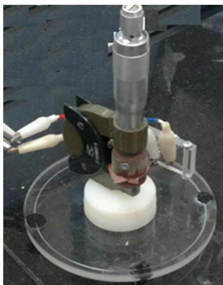
Fig.3. Cell used for measurement dielectric of biological liver tissues
