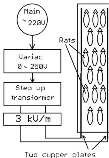
Fig. 1. Schematic diagram for exposure facility system
