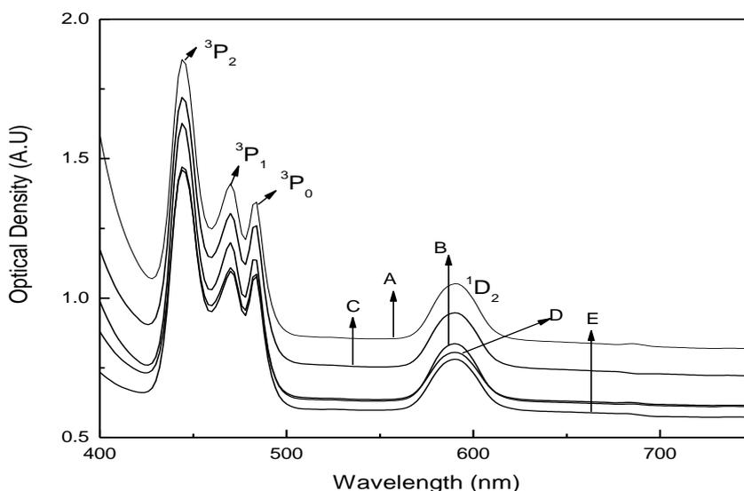
Fig-1 (a) Optical absorption spectra of  $\text{Pr}^{3+}$ : BZCAP 1-5 glasses
