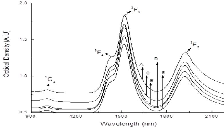
**Fig-1 (b) Optical absorption spectra of Pr<sup>3+</sup>: BZCAP 1-5 glasses**
