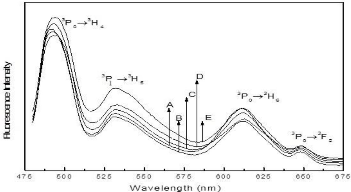
Fig.2. Emission spectra of  $Pr^{3+}$ : BZCAP 1-5 glasses
