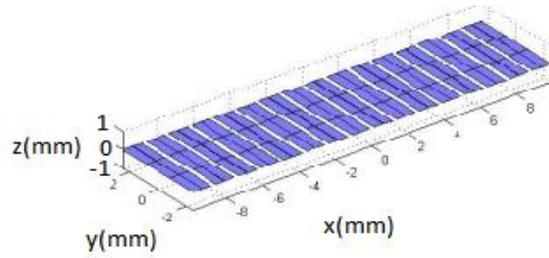
Fig.1 Design of linear array transducer (Height=5mm, Width=0.2mm, Kerf=0.02mm)
