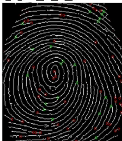
(f) After removing false minutiae (Terminations: 63, Bifurcations: 21)
